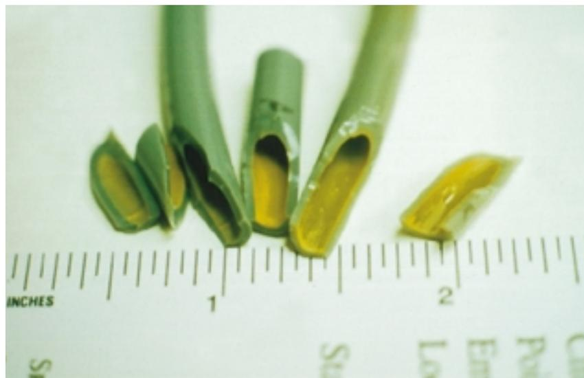
**Figure 3. Biofilm formation on dental unit waterline tubing after six weeks of exposure to tap water. (Photo courtesy of Richard Karpay, D.D.S.)**
